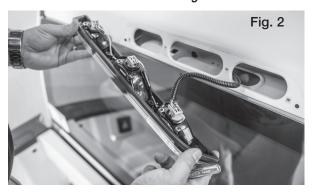
4. With the 3rd Brake Light Assembly removed, position the Main Plate on the truck, check all hardware clearances and shim/adjust as necessary.
