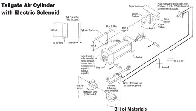
This kit and/or cylinder is designed to allow remote cab opening and closing of the tailgate locking mechanism on a dump body.
