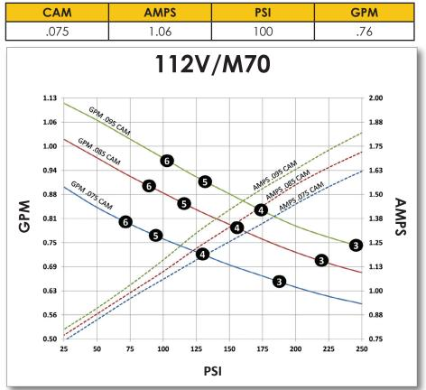
Data recorded pumping water at room temperature and 115V AC power. Actual performance will vary with voltage, application, and mfg tolerances Copyright Pumptec, Inc. 2014
