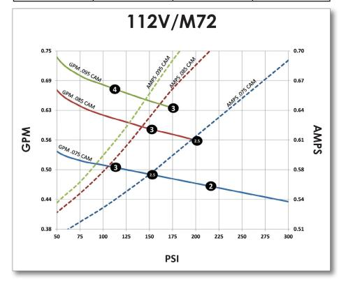
Data recorded pumping water at room temperature and 230VAC 50Hz power. Actual performance will vary with voltage, application, and mfg tolerances. Copyright Pumptec, Inc. 2014
