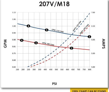
Data recorded pumping water at room temperature and 115V AC power. Actual performance will vary with voltage, application, and mfg tolerances. Copyright Pumptec, Inc. 2014 230V CHART CAN BE FOUND @ WWW.PUMPTEC.COM
