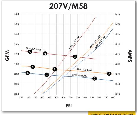
Data recorded pumping water at room temperature and 115V AC power.
